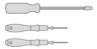
To attach the shoulder mount kit to your URSA Mini you will need a large flat head screwdriver, a 3/16" hex key driver for the top handle and a 2.5mm hex key driver for the Viewfinder adapter plate.
