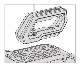
Fasten the handle to any two of your URSA Mini's top 1/4" mounting points using the two supplied 1/4" screws with a 3/16" hex key driver. URSA Mini's rear two mounting points are recommended for most situations, but you can choose any pair for better weight balance when using large lenses.
