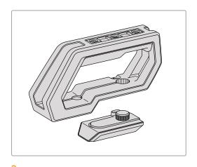
Remove the URSA Viewfinder cap from the base of the handle by gently lifting its arm away from the side of the handle and pulling the cap from the hole.
