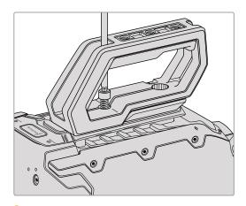
Tighten the screws until the handle is firmly in place and the screws won't easily loosen. Avoid over-tightening the screws as it may damage the screw threads.
