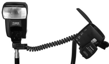
Maximum range, OC-E3 cord with added ferrite clamp
