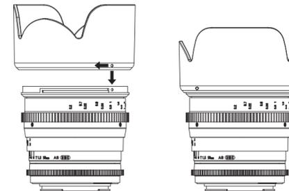
Align the attachment reference point on the hood with the reference point for a hood on the lens, push the hood onto the lens and turn the hood clockwise until it makes a clicking sound.
