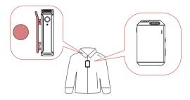
**Note**: Placement of the transmitter in different positions will result in recorded sound volume fluctuations. Avoid any obstructions of the transmitter during recording. It is recommended to use the furry windshield to prevent audio interference when using the transmitter outdoors.
